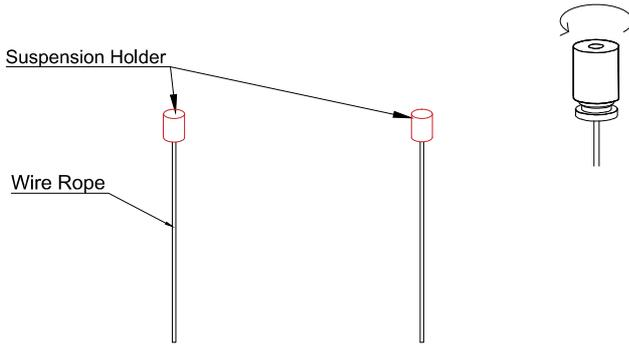
1 Dismantle the suspension holder from the wire rope.
