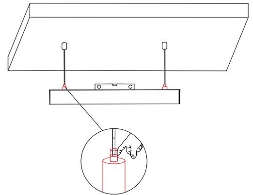
5 Press and hold the gripper of the lower part of the suspension to fix the aircraft cable in place. Make sure the fixture is straight before cutting the excess aircraft cable.
