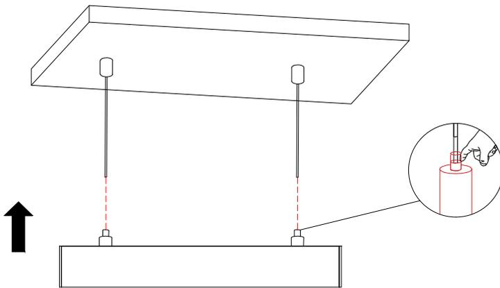
4 Lift the profile than insert the wire rope in the gripper.
