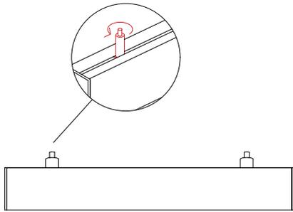
4 In case of need to change the gripper location untightens and slide it.
