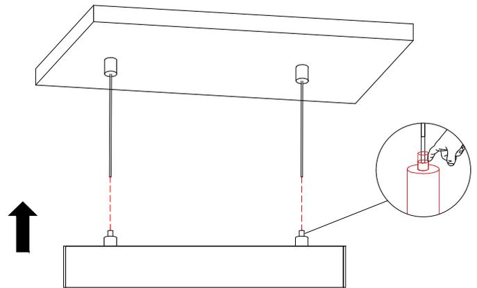
5 Lift the profile than insert the wire rope in the gripper.
