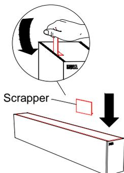
1 Use the scrapper to remove the diffuser.
