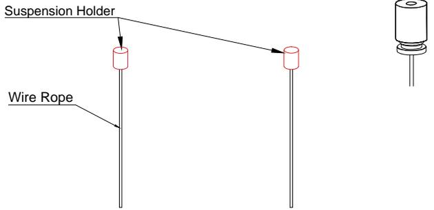
1 Dismantle the suspension holder from the wire rope.
