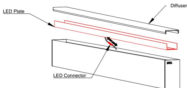
2 Pull the LED Plate and detach the LED connector.
