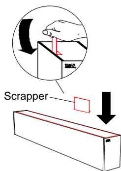
1 Use the scraper to remove the diffuser.
