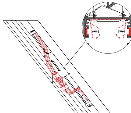
\* Apply silicon on the edges of the profile after joining them to fill all gaps and remove light spill.
